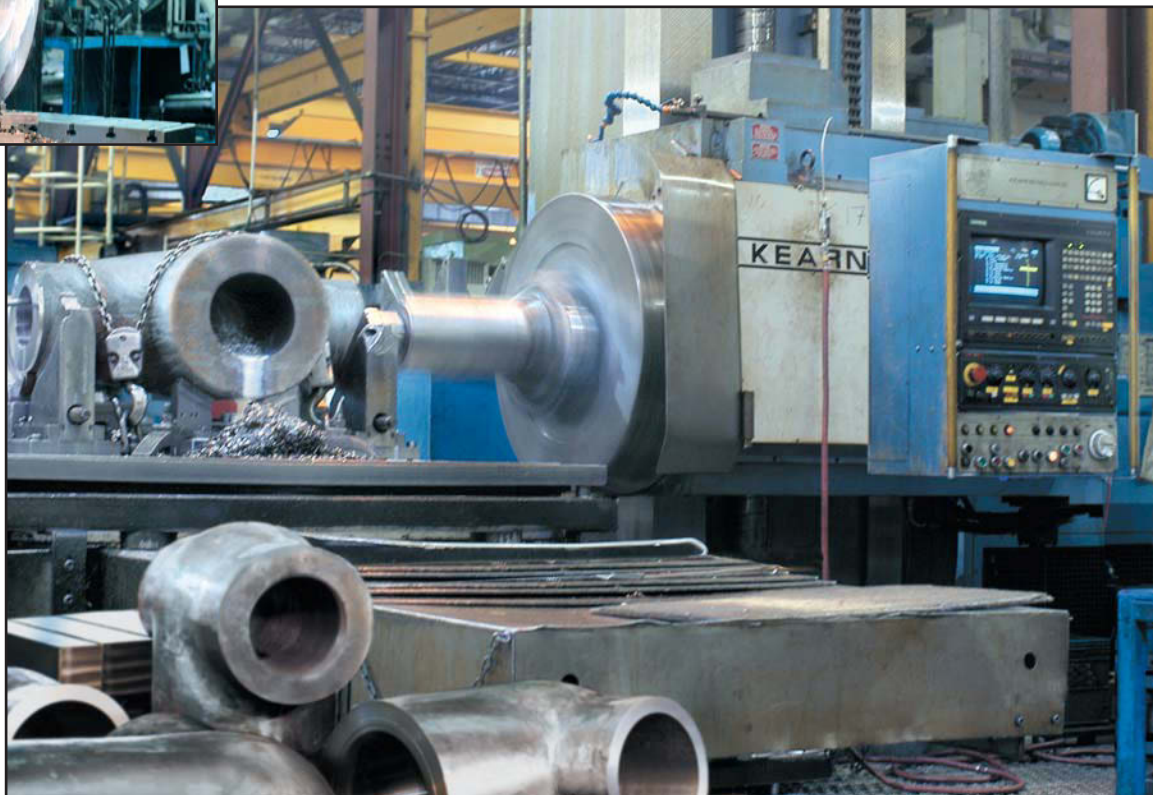
A large CNC horizontal boring mill (with tool changers) machining forged pressure seal bodies.
